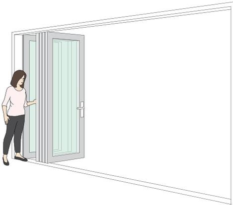
Gently push on the stacked panels while ensuring the access panel is folded flat against the nearest panel.
